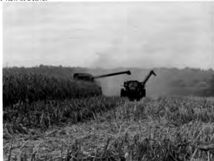
The grain buggy pulls along side the combine ready to receive corn from the combine. In this fashion the combine does not have to stop and can continuously harvest until the field is picked. (photo by Jon Seymour)
